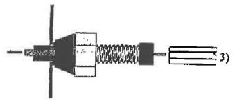
Turn nut the required number of turns - or until firm resistance indicates a complete upset of the BNP.
