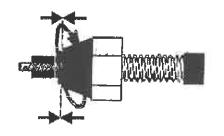
Place hex wrench in socket of jackscrew and hold stationary. Turn hex nut in clockwise direction with a wrench while holding tool at right angle to the work.
