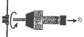
Remove tool from BNP by revolving entire tool in counter clockwise direction.
