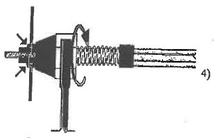
Break nut loose with counter clockwise movement. Remove both wrenches from the tool.
